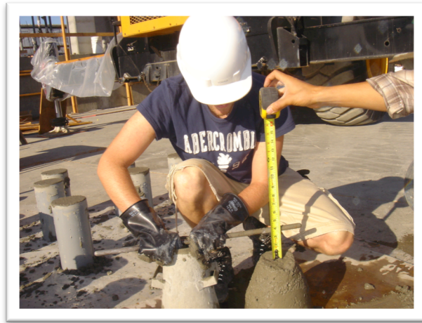
Figure 5 Performing a concrete slump test.
