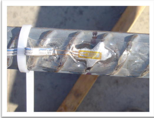
Figure 6 Strain gage in grinded rebar.
