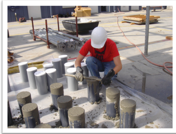
Figure 4 Preparing 6in X 12in test cylinders.
